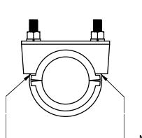
NOTE: - Ensure equal amount of space on each side before tightening U-Bolts . - Ensure equal number of threads on each side of U-Bolt.
